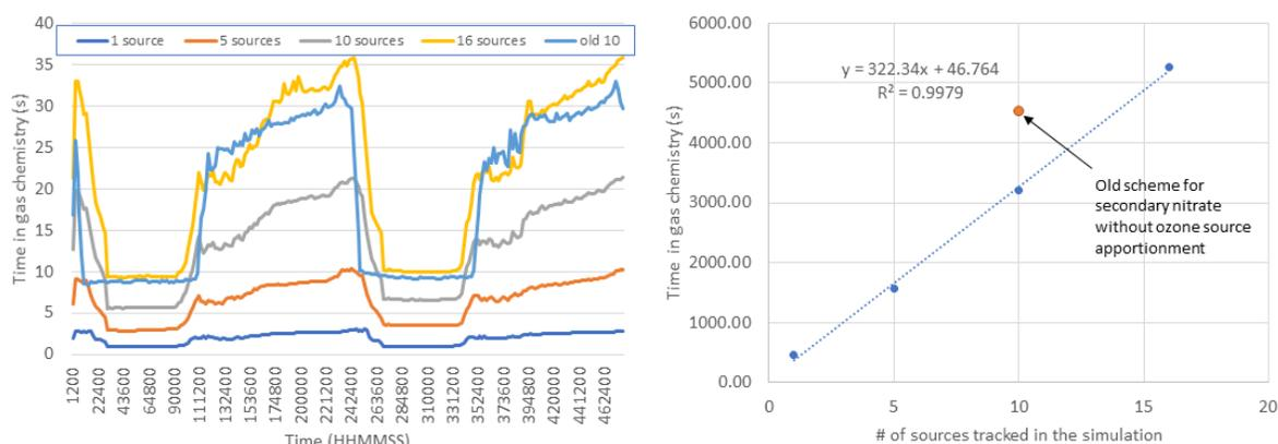
**Figure 1(a)** Wall-clock time for gas phase chemistry at each time step during the two-day simulation (August 28-29, 2006) for simulations with a different number of sources (including the vanilla type) and (b) total wall-clock time for the gas phase chemistry part of the two-day simulation. Units are seconds. All simulations were performed on a 10-core/20-thread E5-2670 v2. Only 8 cores were requested for these simulations.
